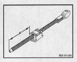
Run the nut onto the screw so that the end of the nut is 90 mm from the cable end of the screw (A).
