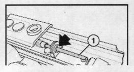
Remove the drive cable (1) from the gearbox and stick it through the guide hole in the rail. Install the screw assembly into the rail and use the drive cable to guide
