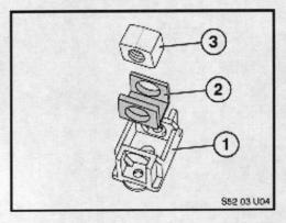
Remove the center section (3) and the isolator pad (2) from the nut assembly (1). Install the new isolator pad and reinstall the center section of the nut. Lubricate the adjustment screw with Wurth Glide grease, article number 0893898. Use an acid brush to distribute the grease over the entire surface of the screw threads.
