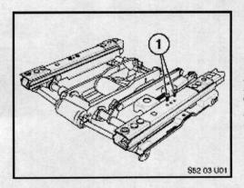
Fasten the anchor nut to the lower rail with two new Torx® screws (1) from the parts kit, and tighten to 4.5 Nm.
