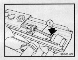
Guide the drive cable (1) back into the gearbox.
