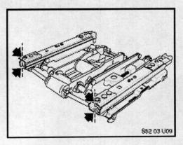
Check the positioning of the upper and lower rails to make sure they are flush. When the procedure is completed on both rails, the alignment of both rails must be identical to prevent binding of the seat when operating. Reinstall the seat.
