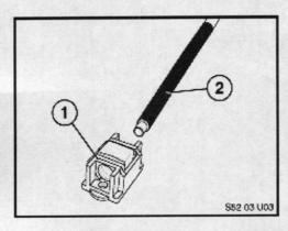
Remove the nut assembly (1) from the adjustment screw (2) and clean off the old grease and dirt from the screw and nut.
