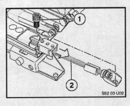
Remove the Torx® (1) screw holding the adjustment screw (2) to the upper rail, and remove the screw assembly from the rail.
