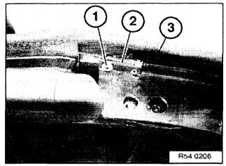
Unfasten screw (1) and remove clamp cable bracket (2).
