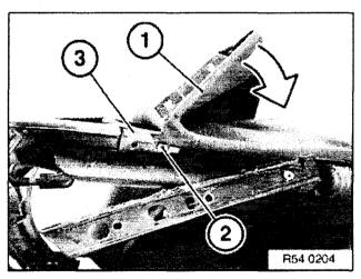
Move front of convertible cover (1) to back. Unfasten screw (1) and unfasten clamp cable bracket (2) from top left/right convertible top linkage.
