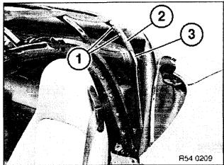
Unfasten blind rivets (1) on clamping cable mount (2) of left/right rear bracket (3).
