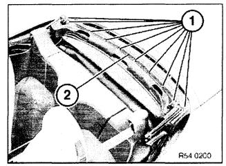
Unscrew bolts (1). Remove frame rail (2) from windshield bracket.
