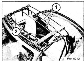
Remove cement residue from the brackets (1) between the clamping straps (2) (clean).
