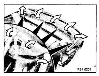
Pull convertible top off cement seal (double-sided adhesive tape, e.g. Tesafix 4965) on front windshield bracket.
