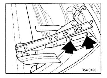
Install side cover mount on windshield brackets at left/right sides.
