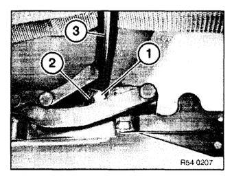
Slightly raise front of convertible cover. Unfasten left/right screw (1) and unfasten side retaining strap (2) on center bracket (3).
