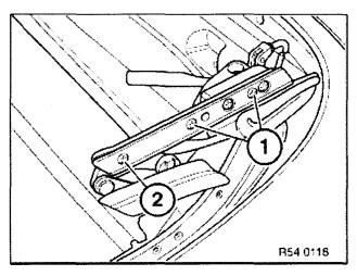
Unscrew bolts (1). Unfasten screw (2) and swivel support rails (for the convertible top gasket) on left/right sides upwards.
