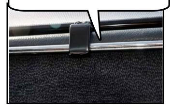
THE FRONT LATCHES ATTACH UNDERNEATH THE CHROME TRIM. UNLATCH THE LATCHES AND LET THEM HANG DOWN
