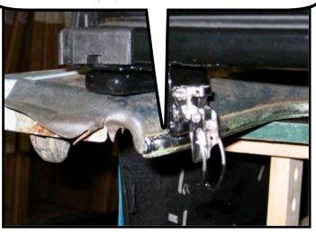
START BY PLACING BOTH LATCHES UNDER THE CHROME TRIM ON BOTH SIDES
