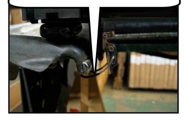
NEXT FLIP THE LATCHES UP ON EACH SIDE SO THEY LOCK THE WIND DEFLECTOR INTO PLACE.
