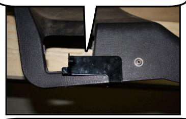
Remove one of the brackets by loosening the large single thumb screw on one end. Then slide the remaining bracket onto the trim panel, close to the middle of the seat belt cover.
