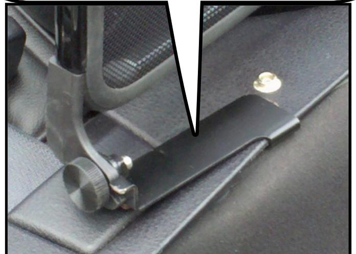
There are two thumb screws that attach the bracket to the trim panel. Start by loosening the thumb screws so there is enough space to slide the brackets onto the trim panel.
