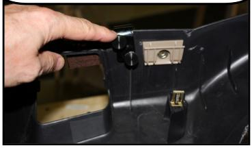
Next slide the other bracket onto the trim panel. Again about in the middle of the seat belt cover, so the wind deflector panel can be reattached to the bracket.
