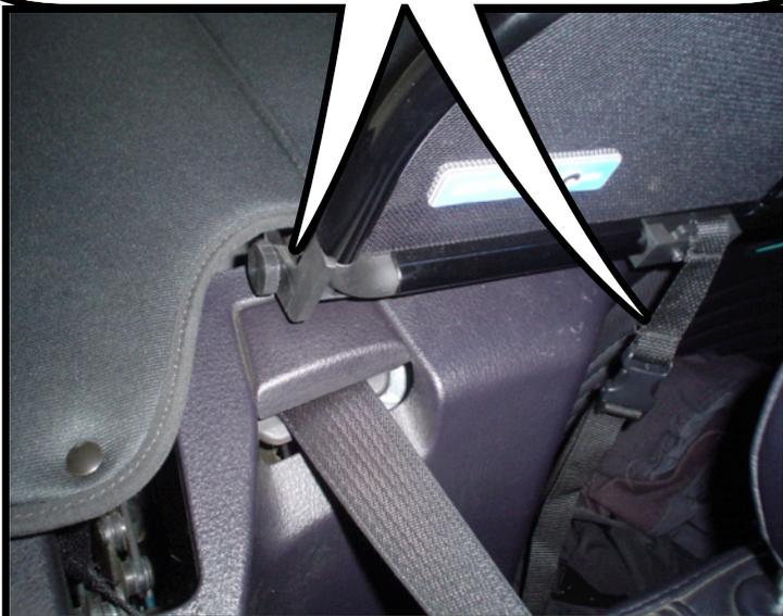
Your wind deflector attaches to your T-bird using two metal brackets and one strap. One bracket on each side attaches to the trim panel behind your seats. The bracket has a felt mat on the bottom so it will not scratch the top of your trim panel.
