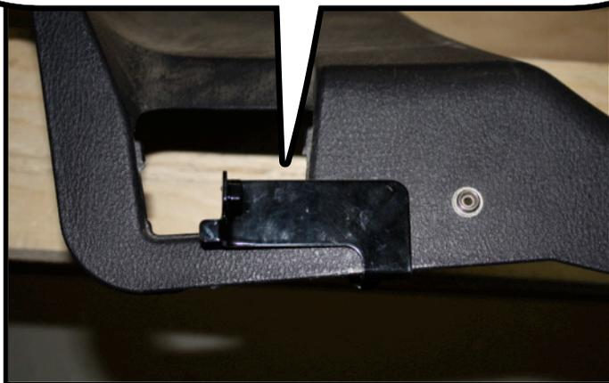
Next tighten the two thumb screws on each side tightly. You might consider using a small pair of pliers. This is a very tight space.
