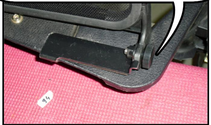
Next slide the other bracket onto the trim panel. Again about in the middle of the seat belt cover, so the wind deflector panel can be reattached to the bracket.
