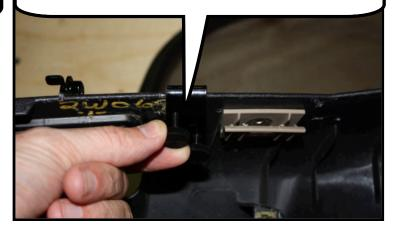
Then attach the large thumb screws on each end to the hole in the wind deflector to the bracket. Now tighten all the small thumb screws.
