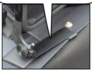
There are two thumb screws that attach the bracket to the trim panel. Start by loosening the thumb screws so there is enough space to slide the brackets onto the trim panel.
