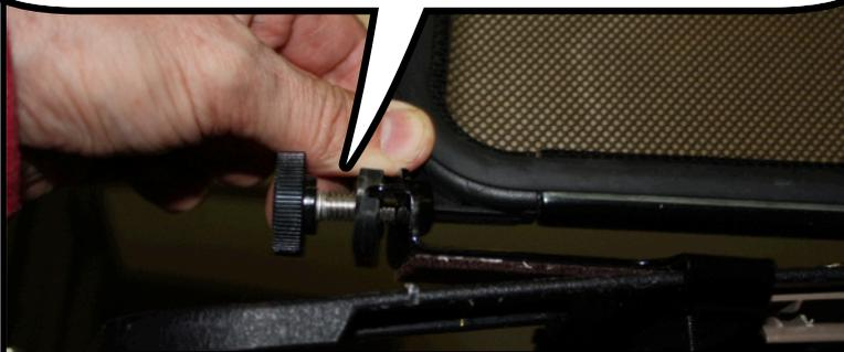
The final step is to attach the snap hook strap to the metal anchor at the bottom of the passenger seat back.
