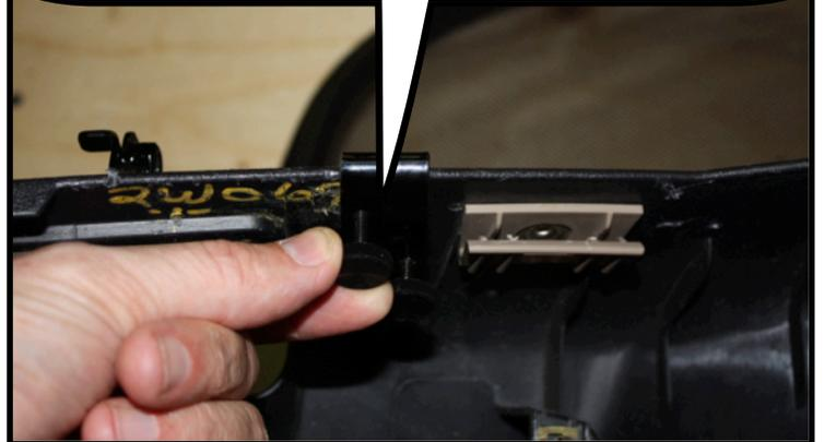
Then attach the large thumb screws on each end to the hole in the wind deflector to the bracket. Now tighten all the small thumb screws.
