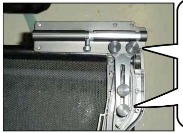
Start by sliding the barrel bolt into the up position. The up position is when all of the thumb screws are below the bolt. Your wind deflector will arrive with the barrell bolts in the up position. Tighten the thumb screws so they are finger tight. The lower position is for storing your wind deflector in your trunk.
