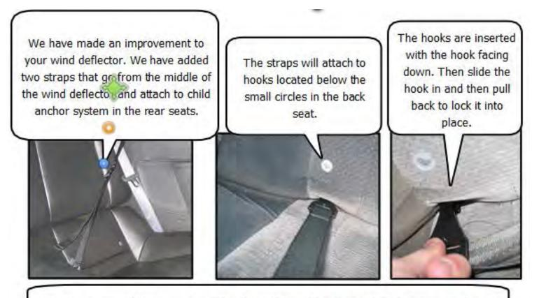
Attach the top and bottom strap and pull to tighten. The straps should be snug so there is no slack but do not need to be very tight.
