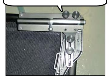
Your wind deflector will fit in the trunk when not is use. Start by folding it up. Then place the locking bolt side in first.
