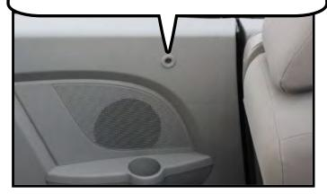
There are also two holes on each side of the rear seat. The holes are about 3 inches down from the top.
