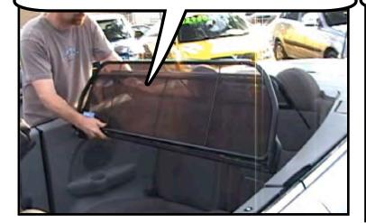
The rear bracket will enter into the holes on each side of the rear trim panel.
