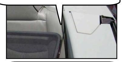
To remove the wind deflector place one hand on each side of the front panel. Note the back hand is not in the same spot as for installation. Now just lift up on the rear of the front panel and the rear brackets will slide out. Unlock the locking bolt on the side closest to you and lift the wind deflector out.
