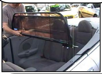
Now on your side lower the wind deflector so it lines up with the hole in the trim panel. Slide the locking bolt into the hole and turn the handle downwards to lock it into place.
