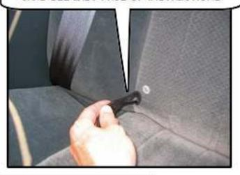
STEP 5 CONT; SLIDE THE BLACK SNAP HOOK INTO THE ANCHOR WITH THE SNAP FACING DOWN. ONCE ATTACHED TO THE ANCHOR PULL ON THE STRAP TO SECURE IN PLACE.
