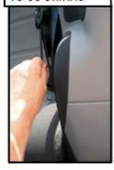
THE FOUR BOTTOM STRAPS WILL LOOK LIKE THIS WHEN ATTACHED. TWO STRAPS GO DOWN FROM BELOW FRONT BRACKETS AND TWO GO DOWN TO THE ANCHOR SYSTEM FROM THE MIDDLE OF THE WIND DEFLECTOR.
