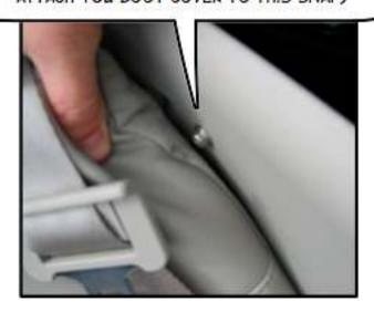
STEP 3 CONT: THE SNAP STRAP IS BEST ATTACHED FROM UNDERNEATH THE WIND DEFLECTOR. ATTACH THE SNAP STRAP ON BOTH SIDES OF WIND DEFLECTOR.
