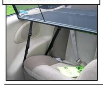
TO REVERSE THE FRONT BRACKETS. TURN THE THUMB SCREWS TO LOOSEN. THEN TURN THE BRACKET TO FACE INSIDE AND REINSTALL THE THUMB SCREWS.
