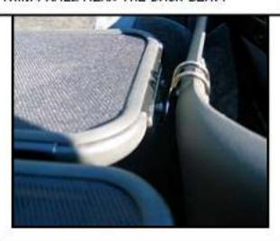
STEP 3 CONT: THE BACK BRACKET HAS A STRAP WITH A FEMALE SNAP WHICH ATTACHES TO THE MALE SNAP ON THE QUARTER TRIM PANEL.
