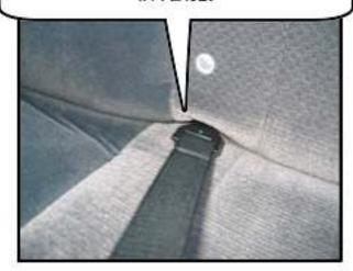
STEP 6: ATTACH THE SIDE STRAPS TO THE BUCKLES UNDER THE FRONT BRACKETS AND THE BLACK SNAP HOOKS TO THE BUCKLES IN THE MIDDLE OF WIND DEFLECTOR
