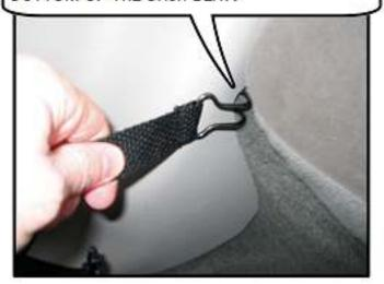
STEP 4 CONT; START BY SLIDING THE HOOK UNDER THE TRIM PANEL AND THEN ATTACHING THE BUCKLE. REPEAT TO THE OTHER SIDE.
