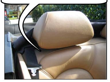
Place the wind deflector into the back seat area. The front brackets will rest on the side trim panel and he rear brackets will rest on the back seat.
