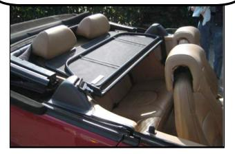
The front brackets sit beside the front seat belt housing. You may need to adjust the front brackets out by 1/8 of an inch, so that the brackets sit firmly on the trim panel. You will only need to do this once.
