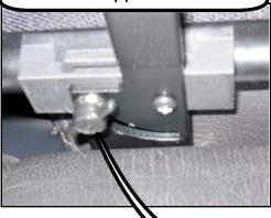
Make sure both brackets are locked into place on the headrest posts.
