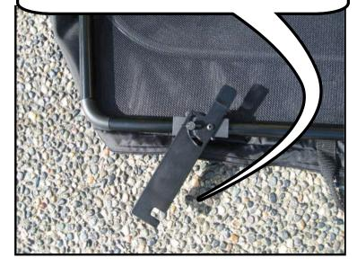
Raise both of the back head rests so that the rear bracket will be able to slide in and attach to the head rest posts.
