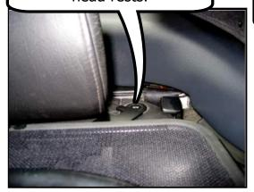
Turn the rear brackets so they lock into the head rest supports.
