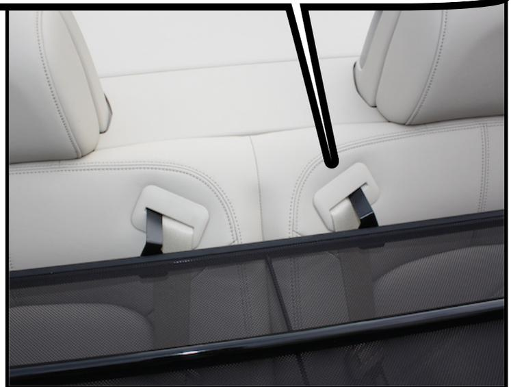
Start by lowering your top and sliding one of the front seats forward. Next align the rear brackets with the slots for the rear seatbelts. Then slide the brackets into the slots.
