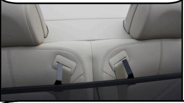
The wind deflector comes with two straps. Attach the two straps with black snap hooks to the Child Anchor system. The Anchors are located at the bottom of your rear seat. Look for to round circles. Slide the hooks in, with the hook facing down, they will lock into place with a snap
