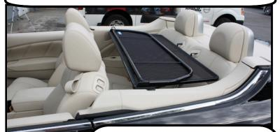
When you need to use your back seat you can put the wind deflector in the trunk. You will need to turn the front brackets so they face in. Loosen the thumbscrews. Turn the bracket around then to insert the screws back into the holes. DO NOT turn them tight
