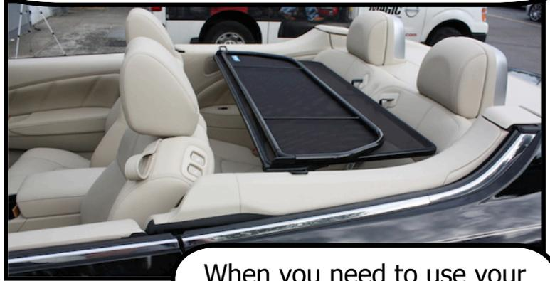
The wind deflector comes with two straps. Attach the two straps with black snap hooks to the Child Anchor system. The Anchors are located at the bottom of your rear seat. Look for two round circles. Slide the hooks in, with the hook facing down, they will lock into place with a snap
