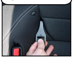
The silver hook straps hook into the bottom of the trim panel and then buckle into the bottom of the wind deflector
