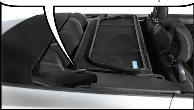
There are 4 straps that hold your wind deflector down. Two use the child anchor system and two attached to the to bottom of the trim panel
