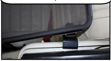
There are 4 straps that hold your wind deflector down. These straps are attached to the bottom of the rear trim panel.
