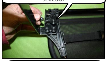
Lay the front brackets flat on the bottom of the wind deflector. The two thumb screws will go into the holes on the on the bracket and into the plastic. The other 2 will go into the plastic.
