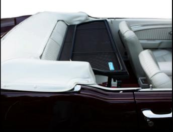
The front brackets are inserted into the Ash Trays in the back seat. Just slide the Ash Tray cover open and insert the front bracket into the front part of the Ash Tray
