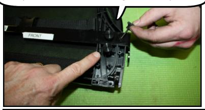
To install the brackets remove the thumbscrews and stand the brackets up. Insert the thumb screws into the holes and tighten. The straight part of the bracket should face towards the rear seat.
