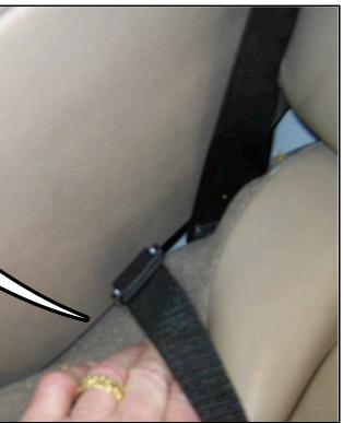
Step 4 Cont: The black snap hook straps then clip into the strap attached at the rear bracket.
