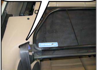
IMPORTANT: NEVER ALLOW THE BRACKET TO SIT ON TOP OF THE SEATBELT AS SHOWN HERE.
