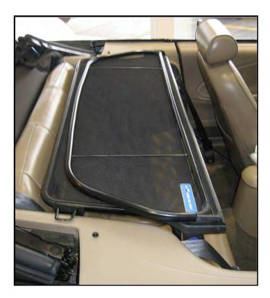
Straps: There are four straps that come with your wind deflector. Two with silver hooks for the front and two with black snap hooks for the rear.
