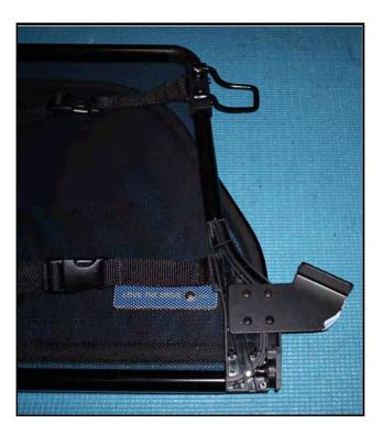
Step 2: You are now ready to install your wind deflector. With the top down, start by placing your hand underneath the front seatbelt strap.
