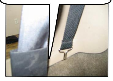
Step 4 Cont: The rear black snap hooks attach to the bottom of the trim panel beside the backseat. There is a small square cut out for the hook. Insert the black snap hook here.
