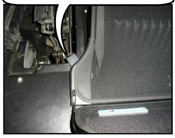
Slide the rear brackets back so that they lock into the trim panel. Tighten the thumb screws on both sides, from the under side of the wind deflector.
