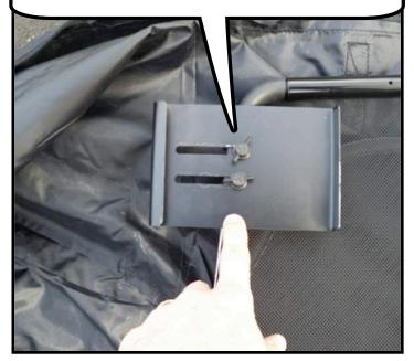
Lay the wind deflector in rear seat area. The front and rear brackets will rest on the trim panel.
