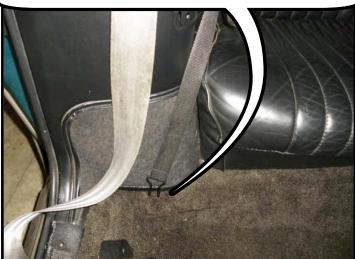
Pull the straps down to tighten on both sides.
