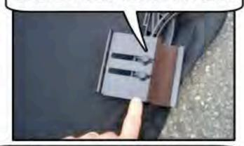
YOUR WIND DEFLECTOR COMES WITH THUMB SCREWS SO YOU CAN ADJUST THE FRONT BRACKETS AS NEEDED FOR YOUR CAR.
