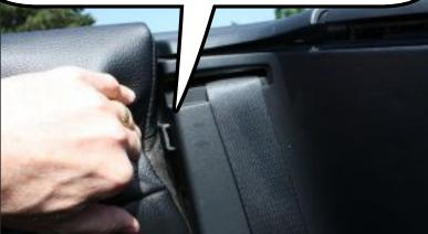
Line up the rear brackets with the bracket holes and then slide the brackets back into the holes
