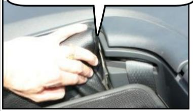
Hold the wind deflector with one hand and lower it so it is even with the rear trim panel
