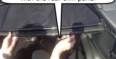
With the handle facing towards the front of the car slide the bolt out and into the hole in the side trim panel.
