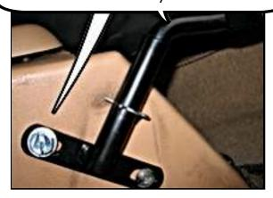
Please note that the tube brackets point toward the back of your Miata. The wind deflector is supported by the shaft bracket and
