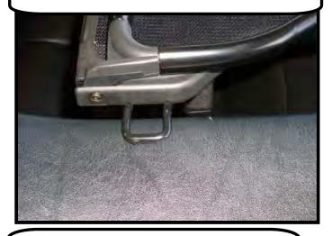
The two brackets should sit flat on the trim panel and not interfere with the rear seat belts.
