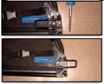
Your Mercedes was designed for a wind deflector. There is a space just below the back seat belts for the rear bracket to sit on.
