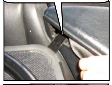
Next attach the silver hook straps to the bottom of the trim panel on either side of the back seats.
