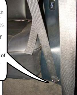
Then attach the two straps to the wind deflector and adjust the straps so they are not loose.
