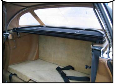
The wind deflector is held in place by two latches on each side and two brackets in the back.
