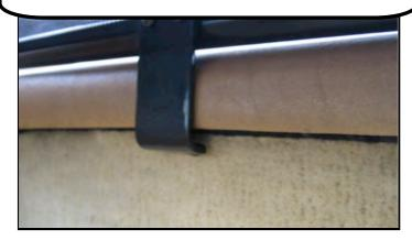
The front latches are located on either side of the wind deflector and latch onto the bottom of the convertible top lid.
