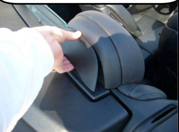
Next, place the wind deflector so it sits on the rear head rests as shown below. Making sure that the black snap hook straps are behind the back seat head rests.
