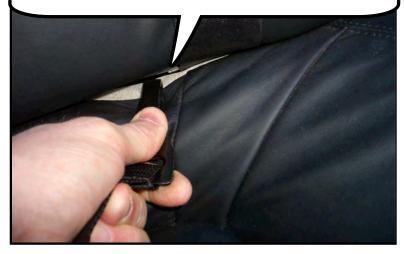
The black snap hooks are inserted with the snap hook facing down.
