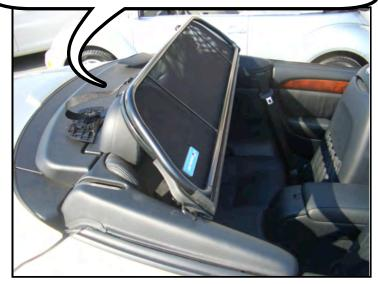
Once attached the black snap hooks will face towards the back of the car. Pull each snap hook up to lock it in place.
