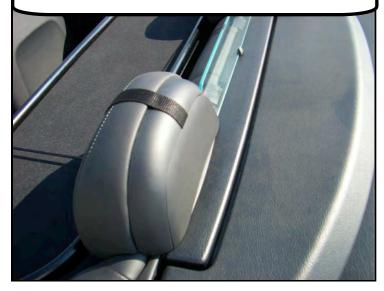
Now lower the wind deflector into the back seat area. The straps attached to the rear head rests will support the wind deflector. The female buckle will hang down into the back seat area.
