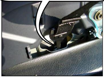
Now attach the black snap hooks to the hole provided from the child seat anchor system on each of the back seat head rests.
