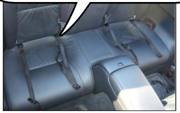
With your free hand push down on the bottom of the rear seat and slide the snap hook in and the down and pull back to attach it to the anchor system. Repeat this step for all four straps.
