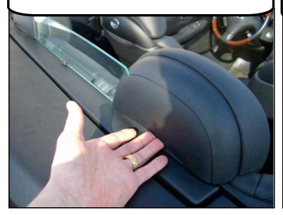
To remove the covers, pull the cover up and back. Behind these covers is a child seat anchoring system that will be used to attach the wind deflector to your convertible.
