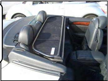
Next you will need to attach the four black snap hooks to the child anchor system in the back seat area. The anchors are located between the top and bottom part of the seat. Look for a small circle child seat logo.
