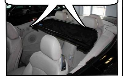
Start by losening the thumbscrews (by one turn) on the rear brackets and turning them so they are at a 45 degree angle like the picture below.
