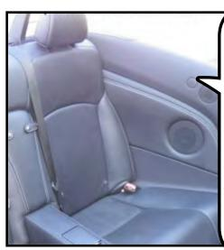
The holes for the barrel bolts may be covered. The holes are underneath the cover just above the rear speakers. If you do not have these covers, you can skip this step.
