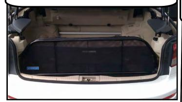
To store the wind deflector, turn handle of the front barrel bolts to the front of the wind deflector and slide back. Then turn the handle down to lock it. Loosen the thumbscrews (towards passenger side) and close the rear brackets flat.
