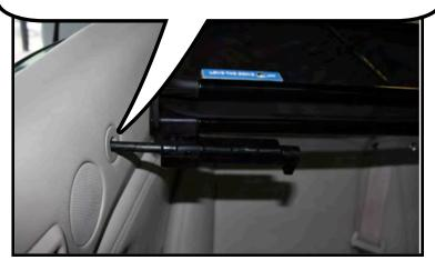
The rear brackets will lock into place around the head rest seat posts. Turning the thumbscrew towards the drivers side will tighten the screws. Turning towards the passenger side will loosen them.
