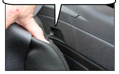
Standing on the drivers side. Flip out the rear bracket on the passenger end. This is what will slide into the slot beside the back seat on the passenger side.
