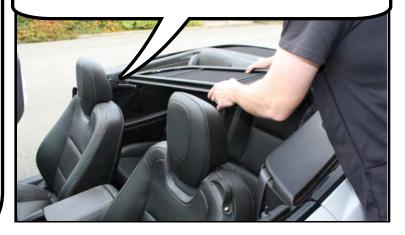
Next, flip out the rear bracket on your end and slide it into the rear slot. Now line up the barrel bolt to the hole in the trim panel, extend the bolt and turn the handle down to lock it into place.
