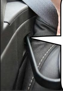
Now lower the wind deflector into the back seat area so the rear bracket goes into the slot beside the rear seat. Then guide the wind deflector so the extended barrel bolt goes into the hole on the passenger side trim panel.
