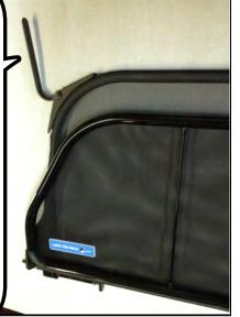
Then extend the barrel bolt on the passenger side as well. And turn the handle down to lock it in place.
