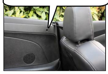
There is also a slot in each side of the rear trim panel beside the back seat. This is where the rear brackets slide into.
