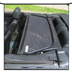
Place the rear bracket behind the dip in the trim panel. Then repeat on the other side.
