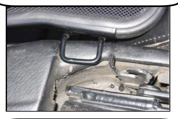
The wire hook when pulled out, will rest on the trim panel just above the seat belt near the front seats.
