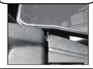
Pull the wire bracket back and forward, then lower it to line up with the space beside the seat belt.
