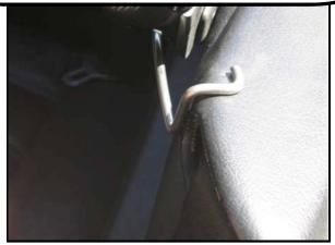
Direct the wire bracket into the space behind the seat belt.
