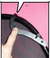
The wind deflector will fit into your trunk when not is use. It is a tight fit. Start by putting the side with the plastic barrel bolts in first. Place one end into the far corner of the trunk.
