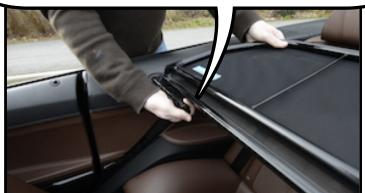
Lower the back of the windstop into the holes between the rear seat head rests. To remove the windstop just reverse the order of the steps.
