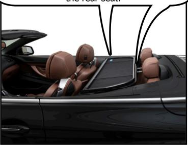
Start by extending one barrel bolt and locking the bolt by turning the handle down.
