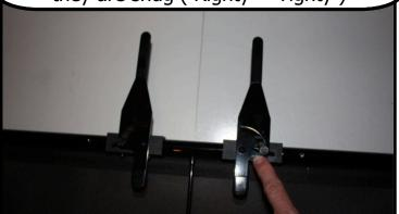
Lower the wind deflector into the back seat. Insert the extend barrel bolt into the hole on the trim panel, on the opposite side from which you are standing.
