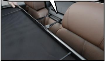
To easily store your windstop in the trunk you will need to lower the barrel bolts. Loosen (do not remove) the thumbscrew at the bottom of the barrel bolt. Remove the top 2 thumbscrews. Slide the bolt down and replace the thumbscrews in the top holes. Reverse the steps to move the bolt to the up position.
