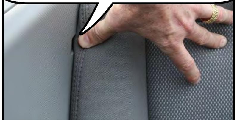
Place one hand on the bottom of the front panel and one hand on the bottom of the back panel.
