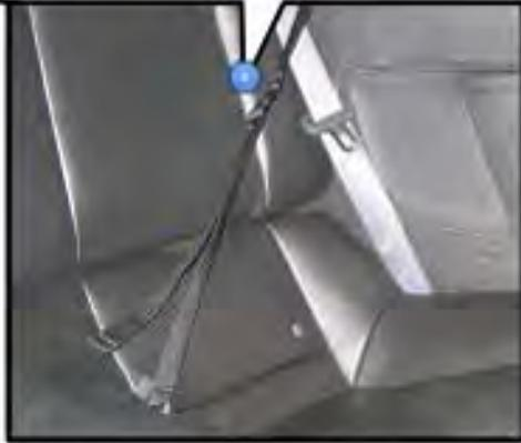
The straps will attach to hooks located below the small circles in the back seat.
