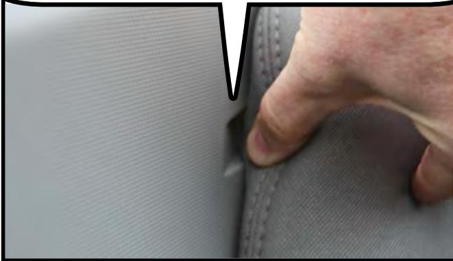
The rear brackets will slide into the holes and the wind deflector will lay flat. The installation is now complete and you can now lift up the top panel.
