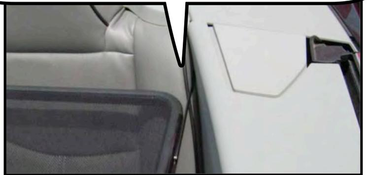
To remove the wind deflector place one hand on each side of the front panel. Note the back hand is not in the same spot as for installation.
