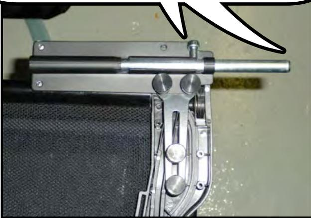
Next lower the wind deflector into the back seat area. Keeping the wind deflector in an upright position as shown below.
