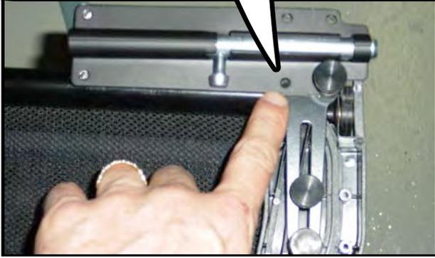
Then slide the locking bolt down, tighten the bottom screws and replace the top screws into the two top holes.
