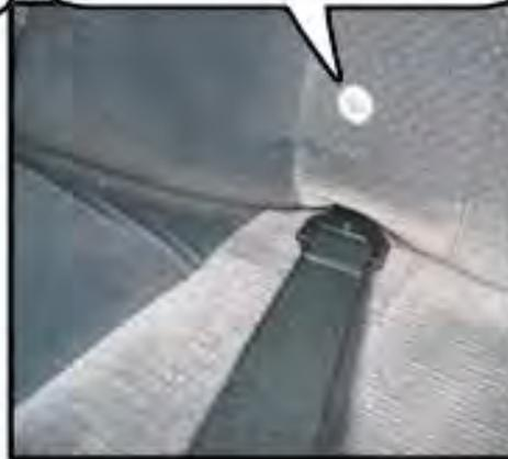
The hooks are inserted with the hook facing down. Then slide the hook in and then pull back to lock it into place.
