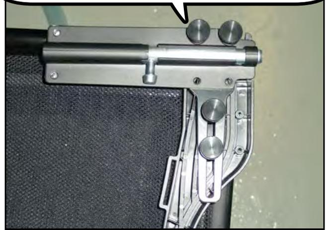
Your wind deflector will fit in the trunk when not in use. Start by folding it up. Then place the locking bolt side in first.
