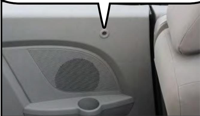
There are also two holes on each side of the rear seat. The holes are about 3 inches down from the top.
