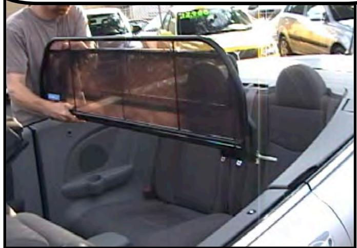
Slide the plastic locking bolt into the hole in the trim panel on the opposite side from where you are standing.
