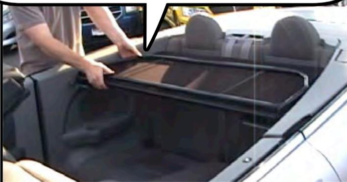
Now just lift up on the rear of the front panel and the rear brackets will slide out. Unlock the locking bolt on the side closest to you and lift the wind deflector out.
