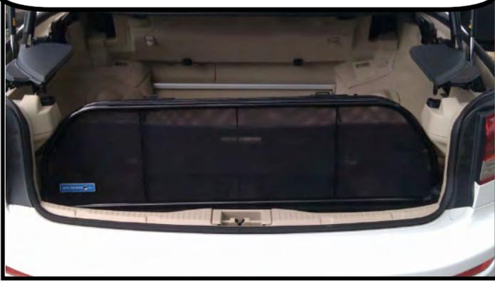
To store the wind deflector, turn handle of the front barrel bolts to the front of the wind deflector and slide back. Then turn the handle down to lock it. Loosen the thumbscrews (towards passenger side) and close the rear brackets flat.
