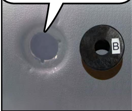
There is a letter "B" on each insert. The letter "B" will point towards the back seat. On the passenger side B will be right side up. On the driver side the "B" will be upside down. But will still be towards the back seat. Tap these in with the palm of your hand or lightly with a hammer. So they are flush to the rear trim panel. You only have to do this once.
