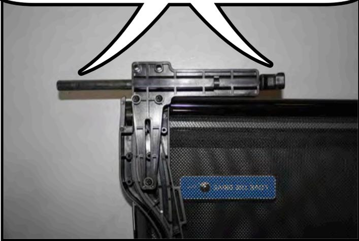
Standing beside the rear seat, lower the wind deflector into the backseat and insert the extended barrel bolt into the hole in the rear trim panel on the opposite side. The rear brackets will rest on the rear seat. Then extend the other barrel bolt into the hole closest to you.
