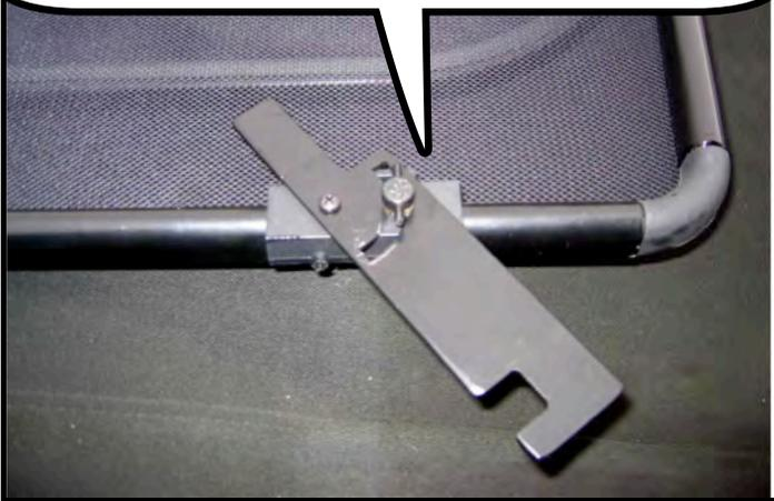
The rear brackets will lock into place around the head rest seat posts. Turning the thumbscrew towards the drivers side will tighten the screws. Turning towards the passenger side will loosen them.
