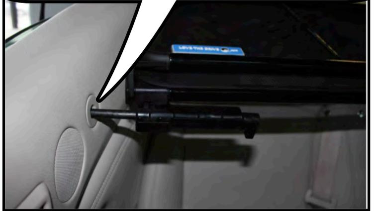
The rear brackets are then turned to 90 degrees so they will lock into place with the rear seat head rests. See next photo.
