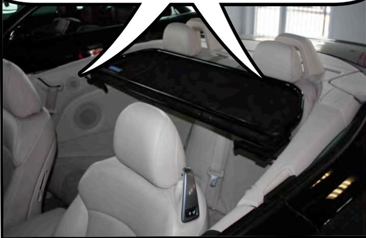
Start by loosening the thumbscrews (by one turn) on the rear brackets and turning them so they are at a 45 degree angle like the picture below.
