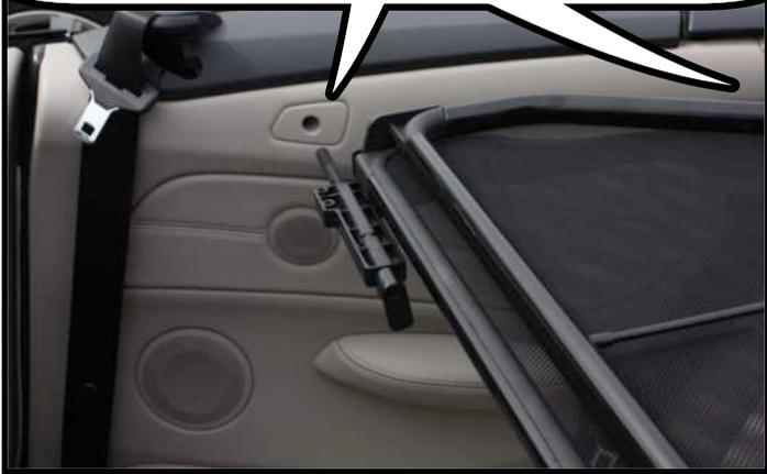
Now lower your end into the back seat area so the front barrel bolt is in line with the front hole. Slide the bolt forward into the hole and turn the handle down to lock the bolt.
