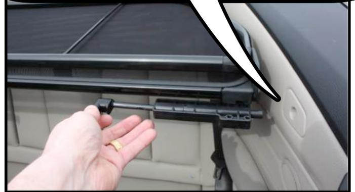
Next reach back and slide the back bolt into the rear hole and turn the handle down to lock the barrel bolt.
