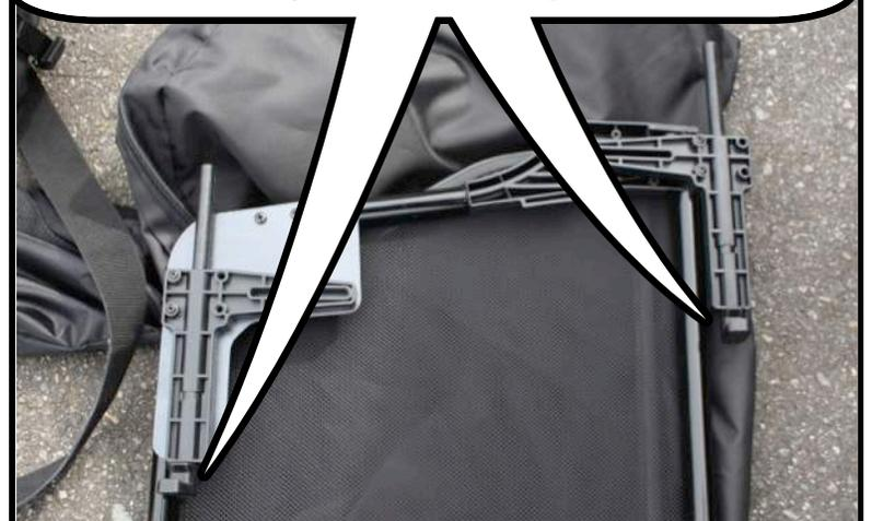
Lower the wind deflector into the backseat area and insert the front bolt into the hole and then the rear bolt.
